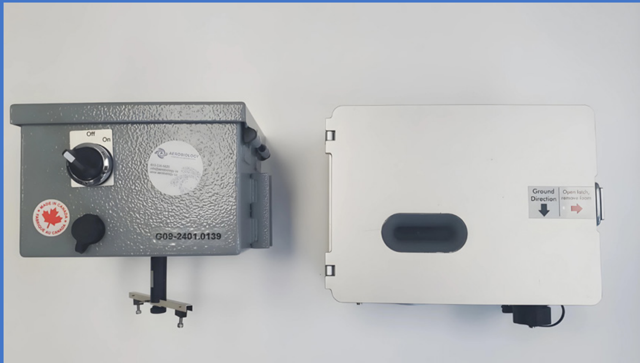
A manual Rotorod Sampler that samples for 24 hours with samples analyzed by microscopy and results available in days to weeks. An automated Pollen Sense Sampler runs continuously with data sent to the 'cloud' and analyzed by artificial intelligence producing data in minutes to hours. Photo credit: A. Johnson, Maine Department of Environmental Protection
