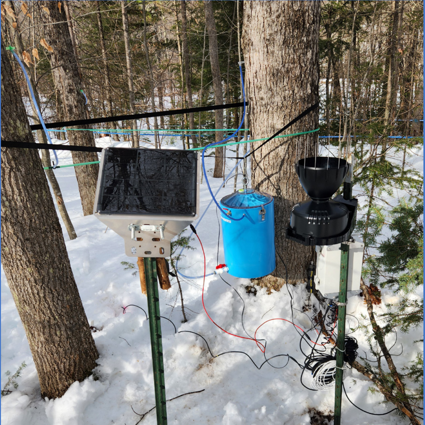
Figure 8. A sensor station monitoring sap flow, internal tree pressure, internal tree temp, soil temp, soil moisture, and ambient conditions in East Dixfield, Maine. Data are being uploaded in real time to a portal used by researchers showing results from a small network of sensors across the maple producing region. (Photo Credit: Jason Lilley, UMaine Cooperative Extension)
